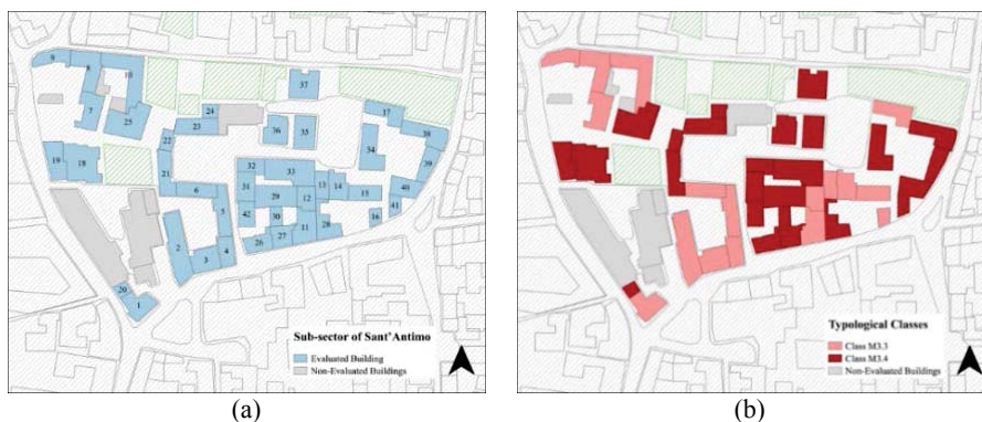
Figure 1. (a) Numbering classification. (b) Typological characterization of the subsector masonry building compounds.
